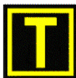
Taxiway Location Sign
